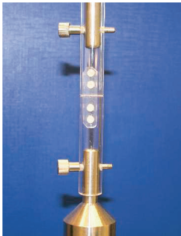
Fig. 3. The test set-up for the tensile test. Please note that the actual tests were carried out in water at 37°C.
